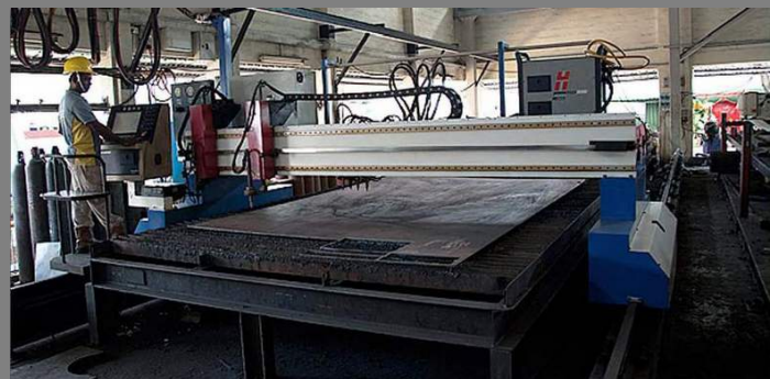
Cutting plates with CNC machine
