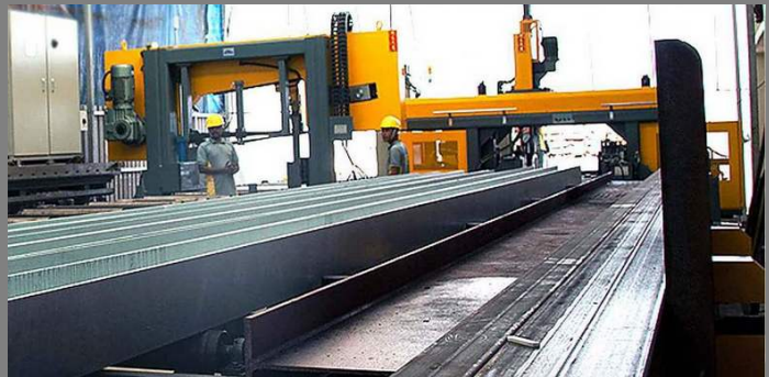
Cutting and drilling beams using CNC machine
